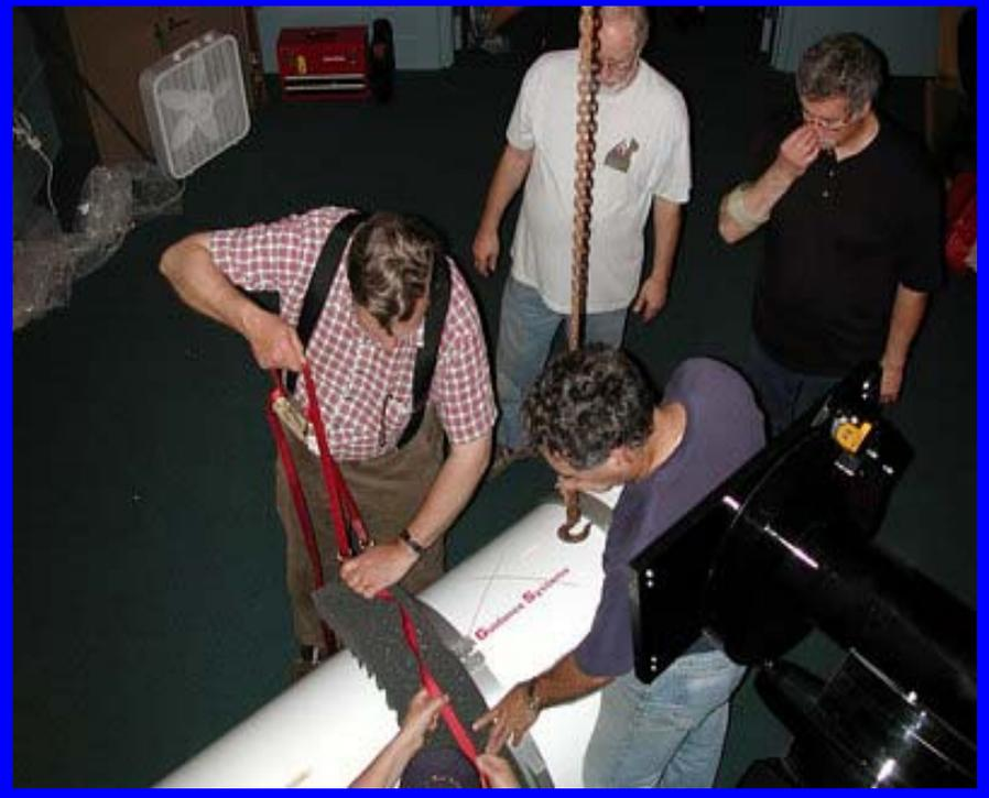
Next we attached straps to the tube in order to raise it by using a come-along attached to the rafters in the roof.
