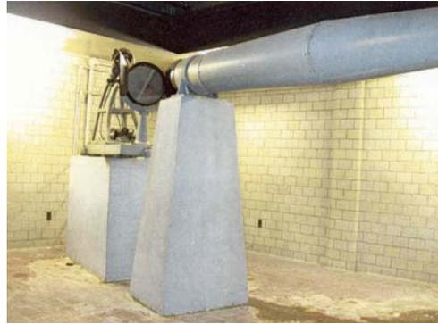
*Fixed Siderostat telescope tube points toward the steerable 10" mirror in this photo from atop the old Buhl Planetarium.*
