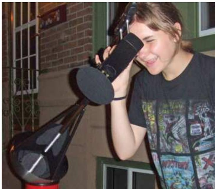
The best part? The mount is rock solid! Even in strong wind, its narrow profile allows the wind to fly by. Its motion, sticktion-wise, was 7/10 until I sprayed a little Sailkote (a dry lubricant) on the bowl. Now I give it a solid 9/10! I'm betting that simple car wax works just as well. You might even find that the original motion is perfectly acceptable.
