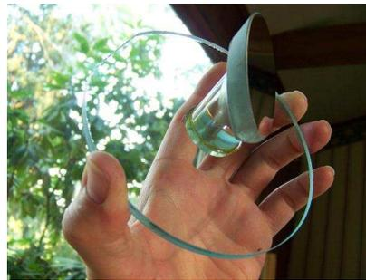
In this image, we see the greenish edge described above indicating that the window is ordinary plate glass. We also see that the diagonal mirror is very nicely attached to the window by a piece of acrylic plastic cut at a 45-degree angle.
