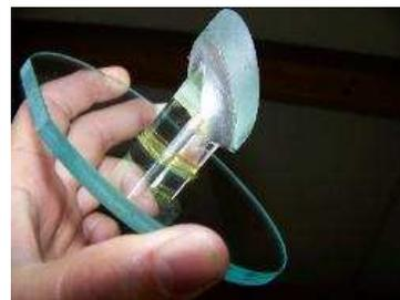
Back view of optical window/diagonal assembly. The diagonal looks to be glued in place.
