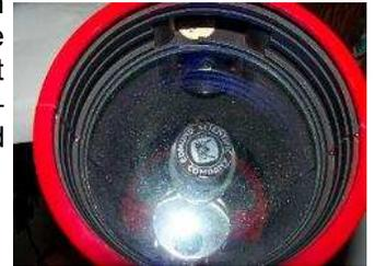
The optical window has become covered with dirt and water spots over the years. The front surface may be cleaned with care, but the inside of the window & diagonal are also in need of cleaning.
