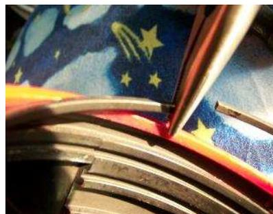
Removal of the snap ring with diagonal pliers
