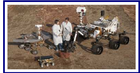
How Martian Rovers have Grown. In the foreground is 1997's 2 ft long Sojourner. On the left is 2004's 5 ft long Exploration Rover and on the right, 2012's 10 foot long Mars Scientific Laboratory Rover
